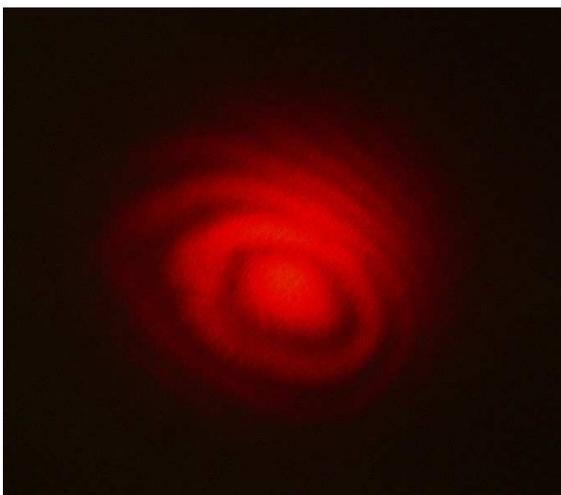
Figure of the interference produced by a red laser by means of the Michelson-Morley experiment. The lighter lines are constructive interference fringes, while the darker lines are destructive interference fringes. Source: Wikipedia
